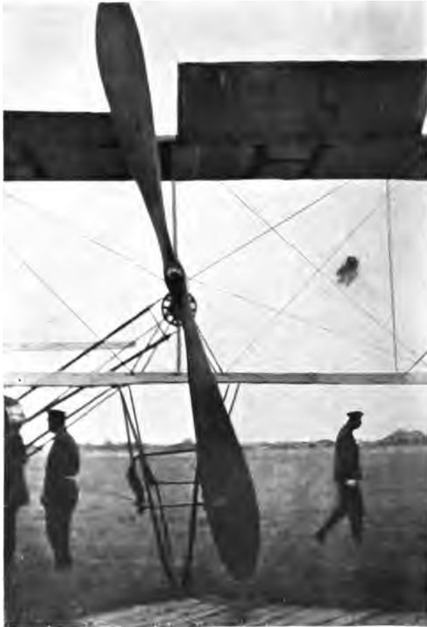
ONE OF THE GIANT AIR-SCREWS OF THE EXPERIMENTAL AEROPLANE "KENNEDY NO. 1," ALTERED CONSTRUCTION, ON THE AERODROME OF THE IMPERIAL ALL-RUSSIA AERO CLUB AT PETROGRAD IN 1914
