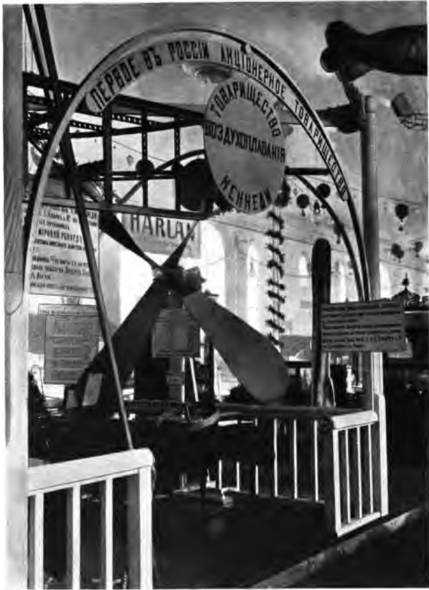
MR. KENNEDY'S STAND AT THE FIRST PETROGRAD INTERNATIONAL AVIATION EXHIBITION, APRIL, 1911. The air-screw shown beat the world's record for efficiency, its co-efficient of efficiency = 81.0 p.c.
